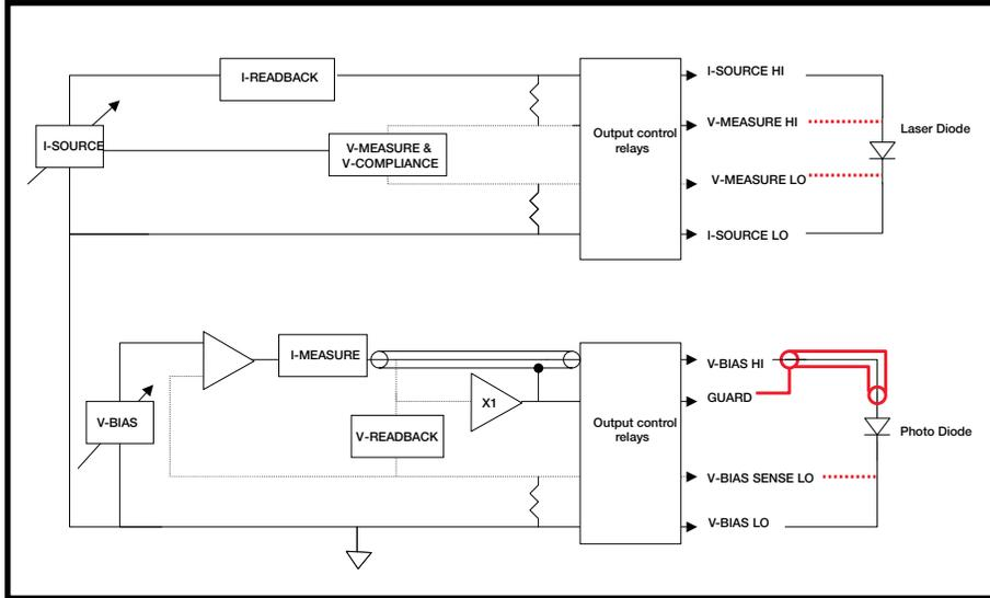
The 450x-QIVC cards incorporate four independent, isolated measurement channels on a single card. Each channel consists of a:
