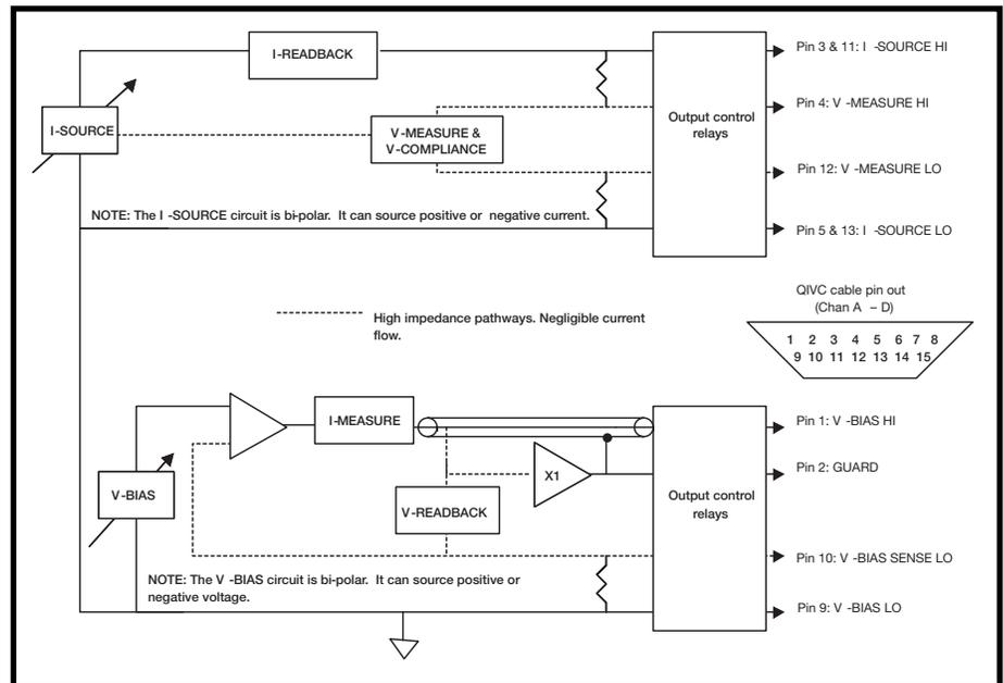
Figure 3. Basic block diagram of source measurement components of the Series 4500-QIVC cards.
